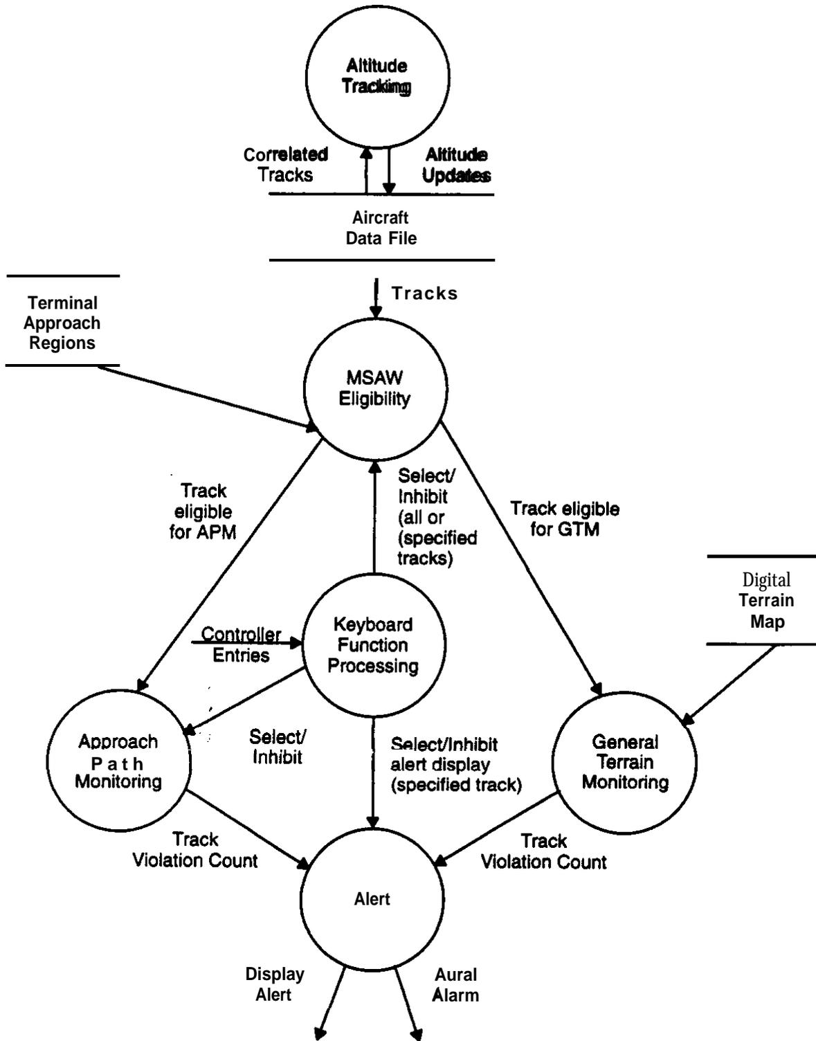
FIGURE 2-1. MSAW/ALTITUDE TRACKING DATA FLOW DIAGRAM
