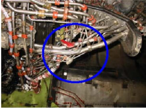
Figure 1.12-13 Bent Pipes, lower drain missing
