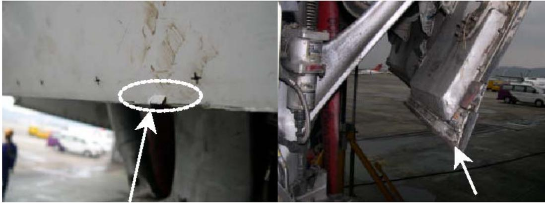
Figure 1.12-4 Deformation and dent to NLG Aft doors
