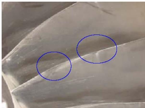
Figure 1.12-12 Fan damage
